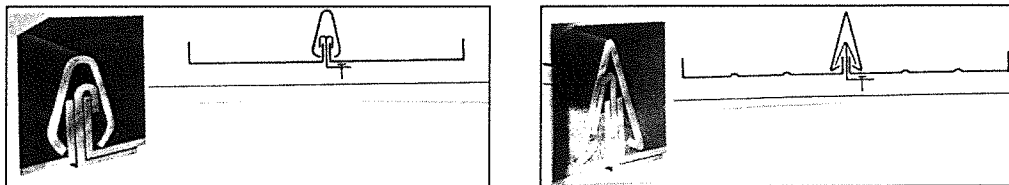
Figure 14.__- __: Low (3/8" x 1") and High (1/4" x 1-1/4") Roof Seams
